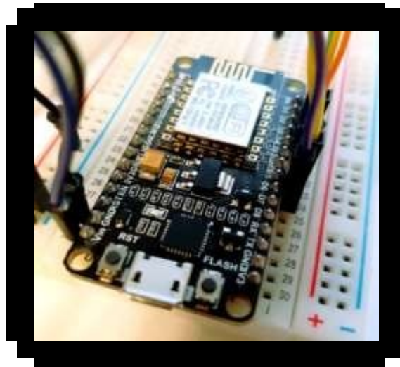
Fig. 5: WiFi Nodemcu module with ESP8266
