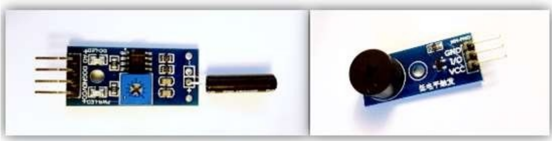
Fig. 13. Seismic Sensor (left) and buzzer (right)
