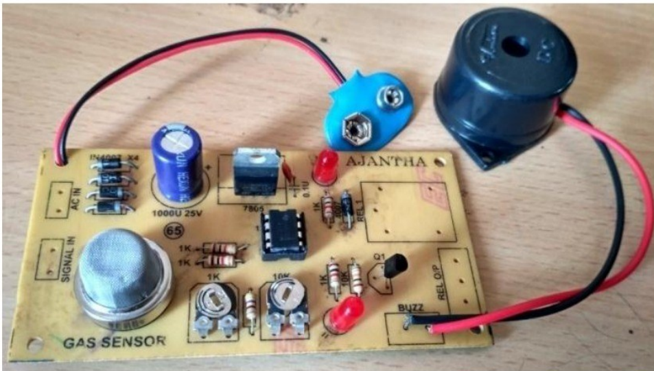
Figure 5: LPG leakage detection and alert system
